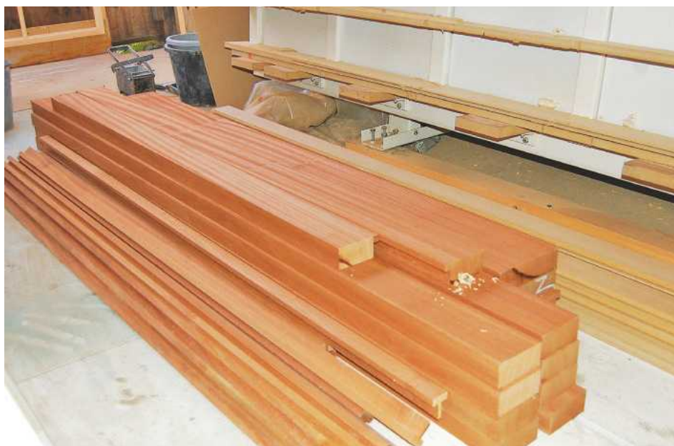
▲ Pic.1 The prepared timber, complete with rebates and planed to size
